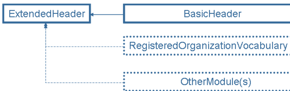
Figure 5 — Extended Header structure
