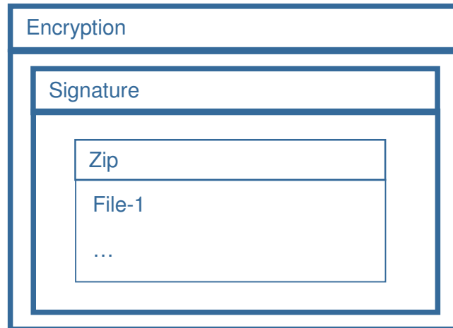
Figure 6 — Layers and structure of a container
